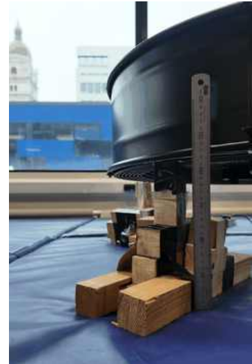
(c) outlet height: 0.425 m, support offset: 0.220 m.
