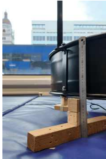
(b) outlet height: 0.330 m, support offset: 0.125 m.
